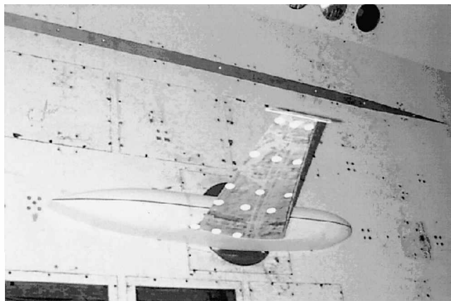
Fig. 1 MAVRIC-I model mounted on tunnel sidewall.
